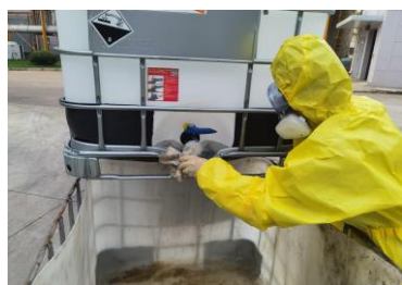
将泄漏吨桶上残留的废液擦拭干净
